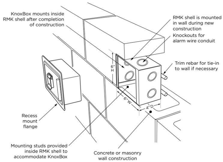
**Recess Mounting Using Recess Mounting Kit**
